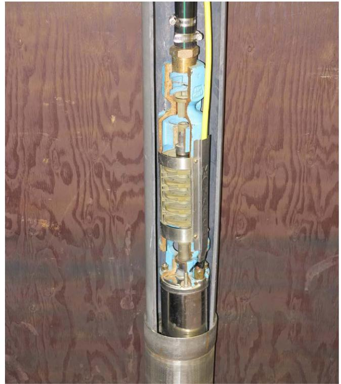
*A submersible pump in a drilled well casing model.*
